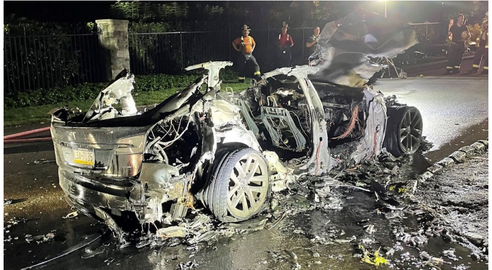
All that remains of a burnt EV is essentially an empty shell that shows that many aluminum body panels melted away. The reignition issue because of stranded energy that's inside of the floorpan-mounted battery remains. Photo from Firehouse Magazine.
